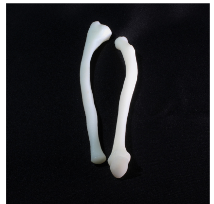
FIG 3 High resolution SLA models of full radius and ulna showing 3D rotation.
